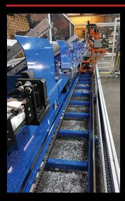
This custom drilling and annular cutting machine makes aluminum parts for a construction-industry brake. It features a single drillhead (orange frame) that travels 16 feet at speeds of up to 2 fps. Photo courtesy Lumco Manufacturing Co.
